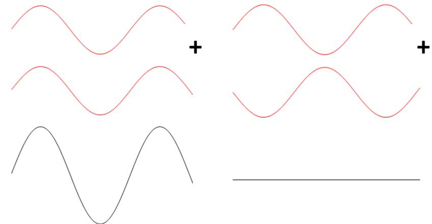
Figure 1 Constructive and Destructive interference
