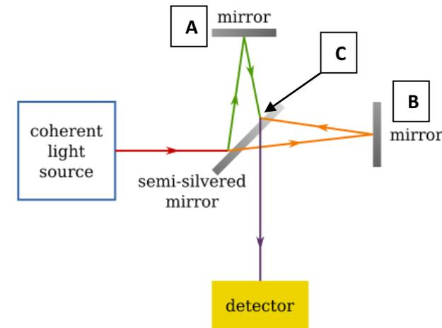
Figure 3 Michelson Interferometer
